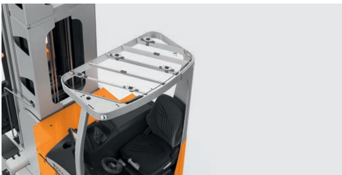
Whatever the application, we offer the right overhead guard, visibility-optimised, with or without metal or polycarbonate cover
