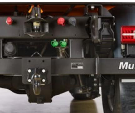
Powerful: the ball head/pin coupling with a drawbar load of 150 and 250 kg respectively.
