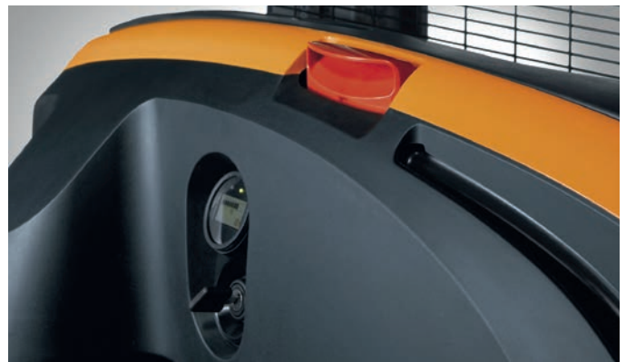
Unauthorised access not possible: access authorisation by key, PIN code, chip or card
