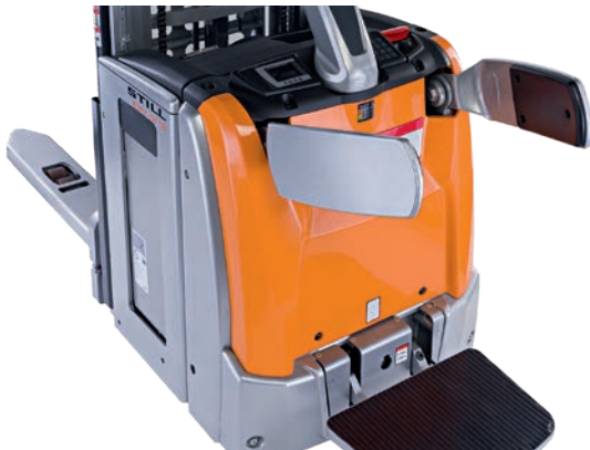
Reduces back strain: air suspended stand-on platform adjustable to the individual weight of the driver
