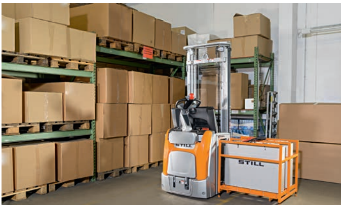
Ready at all times: high availability thanks to optional lateral battery change
